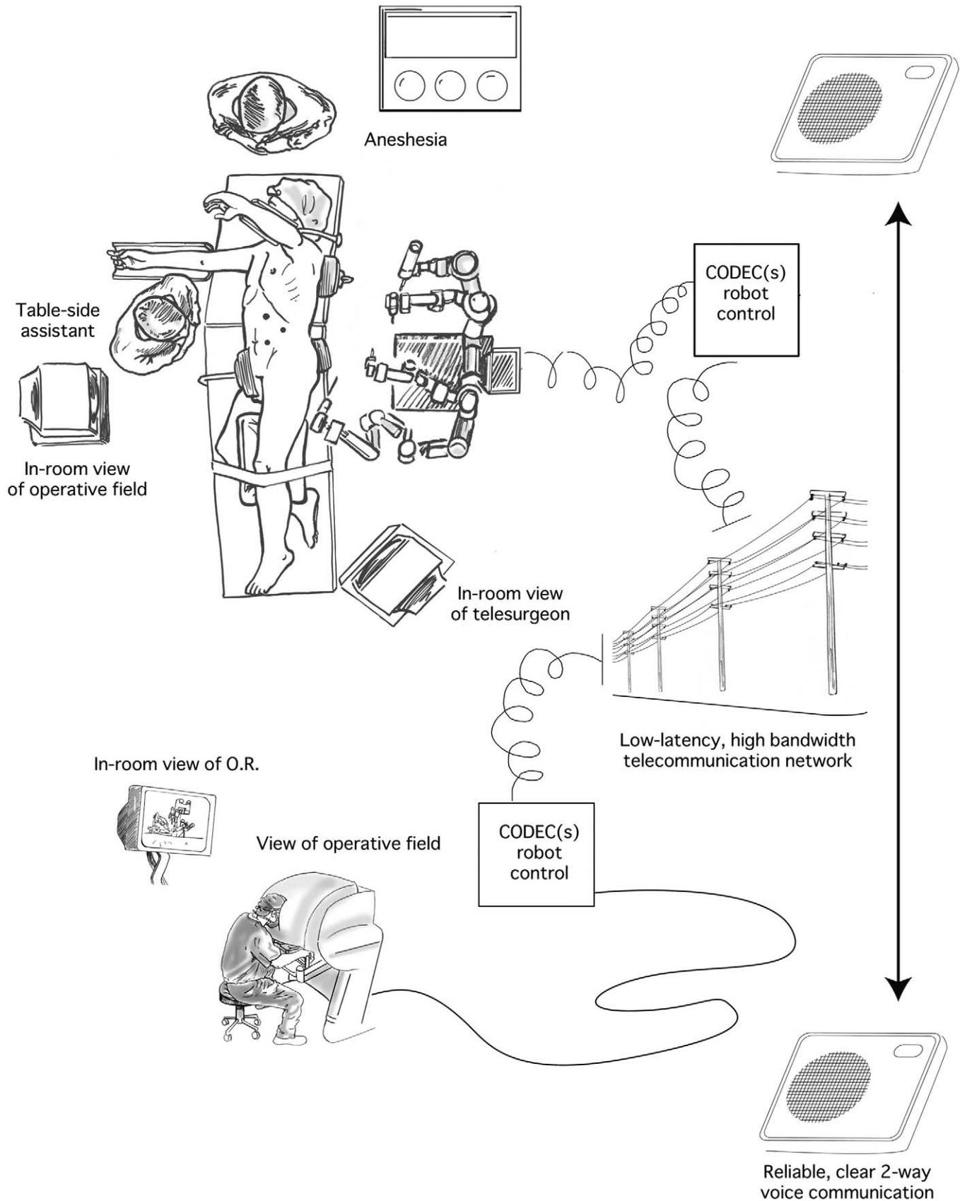
**Figure 3** Essential components of a telerobotic surgery circuit.
