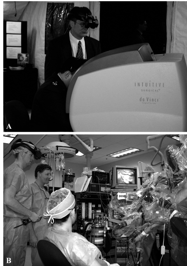
Fig. 1. Telesurgery using the da Vinci surgical system. Surgeons in Denver, Colorado (A) operate on a pig in Silicon Valley, California (B) through the Internet
